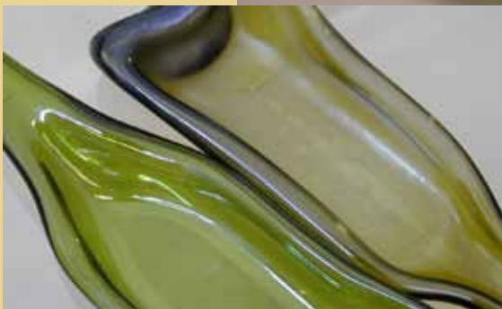
The upper right was fired without any overglaze; the lower left was fired with coat of Fusing Solution.
