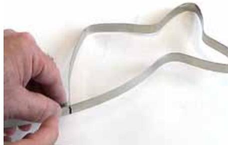
The connecting point is where the two ends of the band come together. It is possible to tack weld or drill and bolt these ends with a stainless steel screw, but the easiest way to secure them is to make a folded tab.
