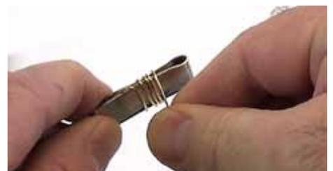
Secure the connection by wrapping brass wire around the combined tails. Your form should now be secure. Fine tune your shape by gently bending the banding.
