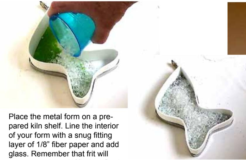
Place the metal form on a prepared kiln shelf. Line the interior of your form with a snug fitting layer of 1/8" fiber paper and add glass. Remember that frit will compress about 50% when fired, so 1/2" thick layer of frit will fire down to 1/4" solid piece of glass. Piling the majority of the frit in the center of the mold will minimize the sharpies around the edge. This sample had over 1" of frit and melted down to a 1/2" thick finished piece of glass.
