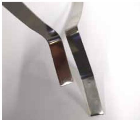
Make two tabs that extend beyond the connecting point. The Short Tab should be about 1 1/2" long. The Long Tab needs to be 3" long or twice as long as the Short Tab.
