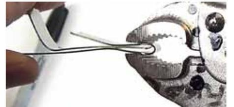
Bend the 3" Long Tab in half. You want it to fold back onto itself 1 1/2" in from the end. Insert the short tail into the gap of the long tail and pinch the long tail as tight as you can with pliers or vise grips.
