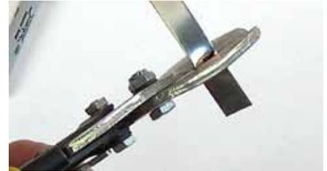
If needed, cut the banding with metal shears or a hacksaw.
