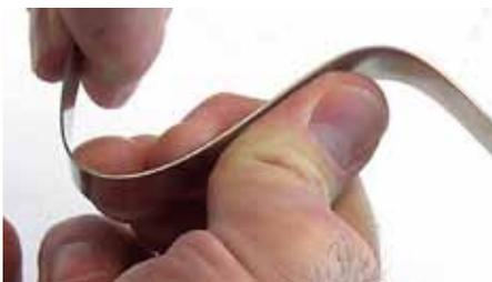
Gently bend the banding into the form you desire. If you are making a circle, it is helpful to wrap the banding around a form. Other shapes can be bent free hand.
